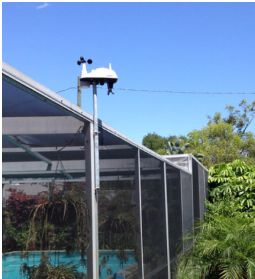
The “Mango” WeatherUnderground station for Gulfport. Well below the surrounding treeline. Useless for sailors.
